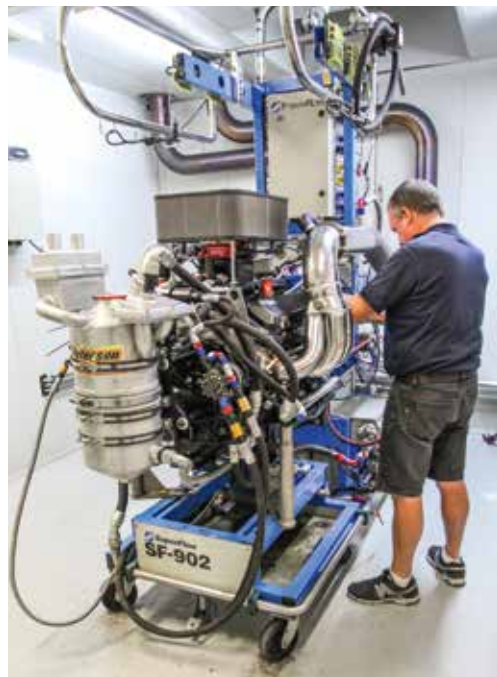
Right: All engines are run on the team's dyno before being installed in the boats.
